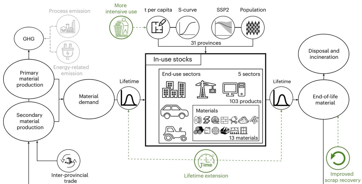
**Fig. 1 | Overview of the IMAGINE Materials model.** IMAGINE Materials: integrated modelling of the material–energy–emission nexus associated with bulk materials. SSP2 refers to shared socioeconomic pathway 2.
